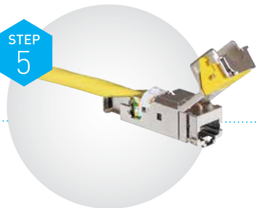
Install the wire housing without pushing
